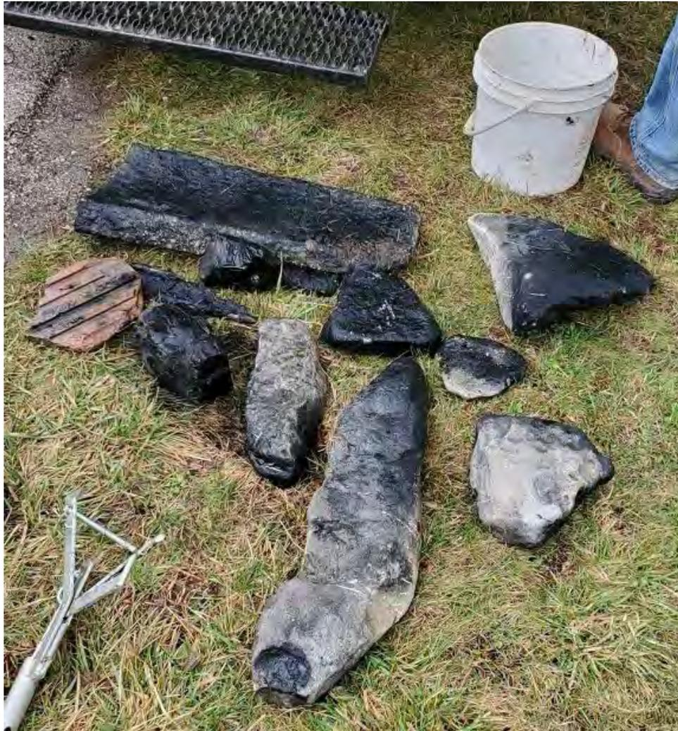
*A sample of material pulled from a single manhole on the 30" interceptor at Cedar Creek (March '22).*
